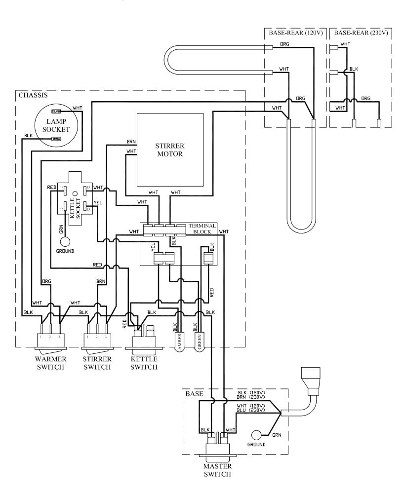
PS/TP-16 WIRING DIAGRAM (120V)
