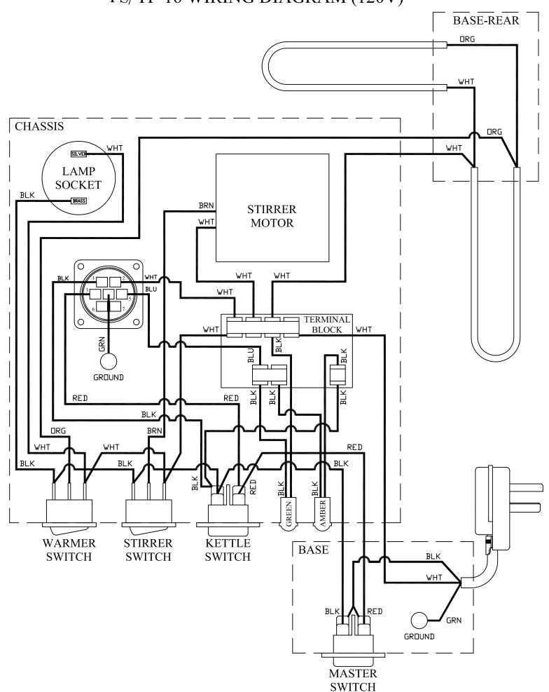
PS/TP-16 WIRING DIAGRAM (230V)
